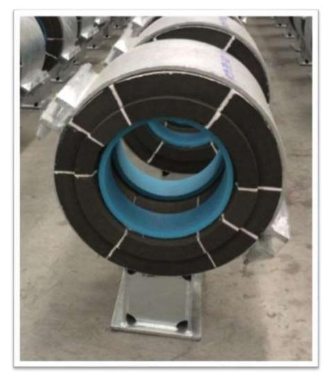
In process plants, pipework sometimes needs to be designed for both cold and hot operating conditions. PUF insulation is not used above about 130°C and calcium silicate is not used below zero. Where neither of these materials meets the required temperature range, the type of insulation most commonly used is Foamglas.
